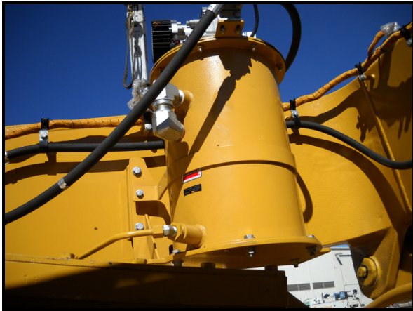
Existing OEM Auto Lube Location
