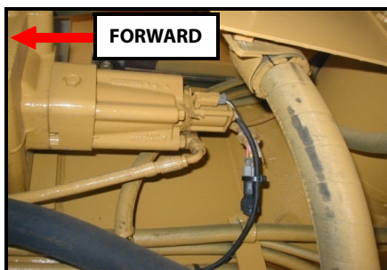
Typical Hoist Valve Wiring
